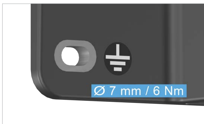
Fig. 5.15: Grounding connection at the left mounting hole
