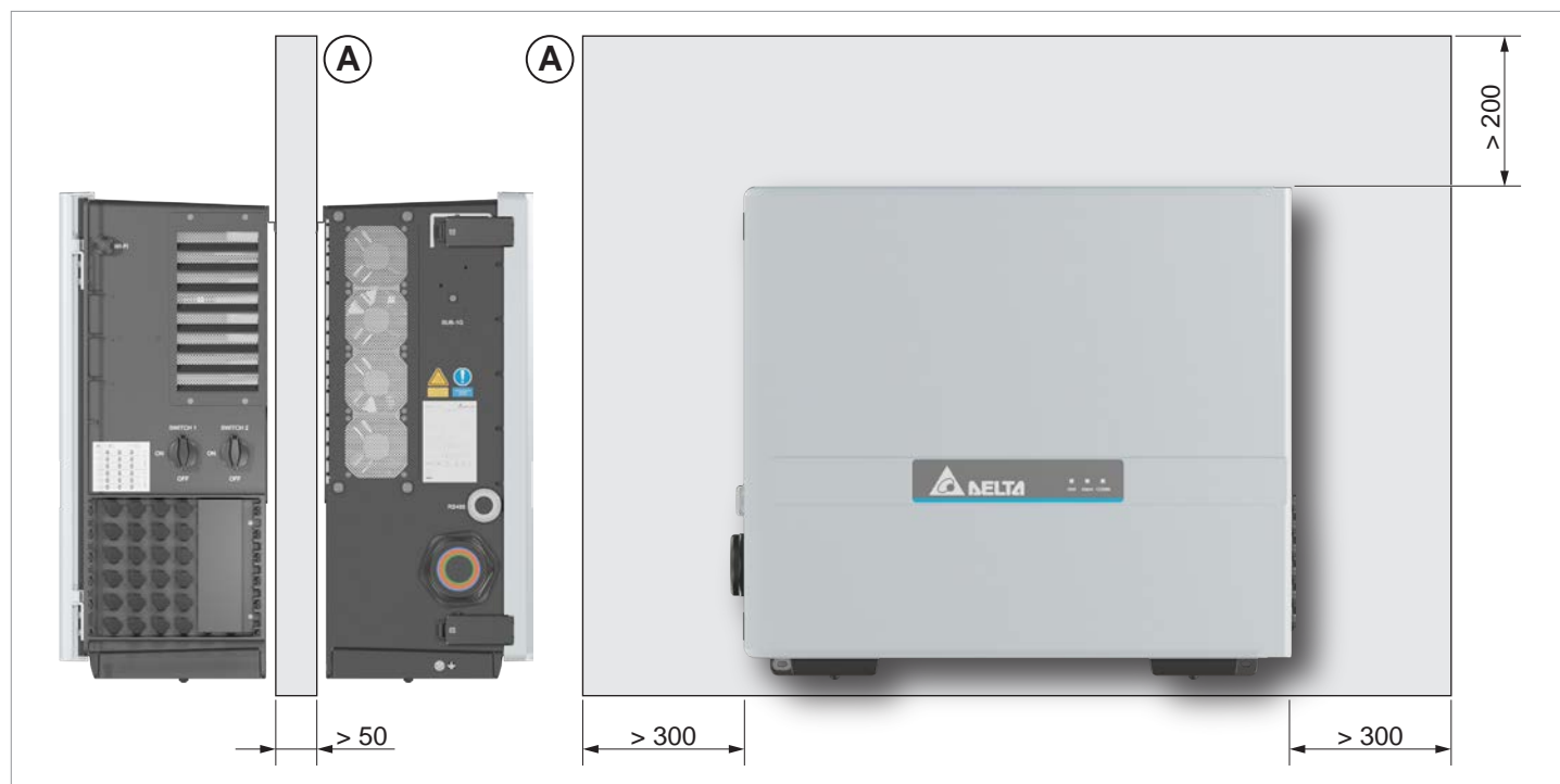
Fig. 5.6: Mounting distances and air circulation, variant 3 (in mm)
