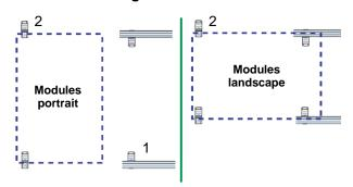
The short profiles with a length of 125 mm are to be placed on the inner side (1) of the top and bottom insertion rail and alternately on the top and bottom (2) of the middle insertion rails in accordance with the static calculation on the high beads and tightened with the required number of fasteners.
