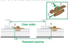
MV 9.2 Position of the cross rail connector IR
