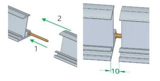
Push the connector into the secured rail piece up to half way into the screw channel, then push the lose rail piece with the screw channel onto the connector with a 10 mm gap between the rail ends, then attach the second rail piece.
