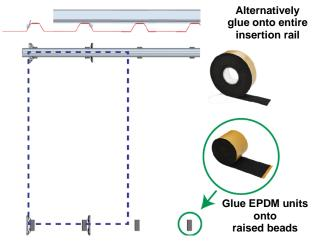
Glue the EPDM units onto every raised bead below the insertion rails. Alternatively, the EPDM tape can also be glued onto the insertion rail for small raised bead distances.
