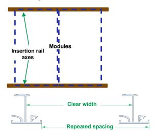
Mark the mounting axes of the insertion rails on the trapezoidal metal raised beads dependent on the module orientation - portrait or landscape.
