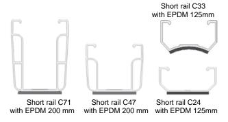
To improve ventilation behind the modules the modules can be mounted using the short rail C47 or C71, the mounting steps must be carried out as described in chapter 5.1.
