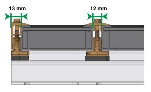
End clamp mounting flush with the rail end possible.
