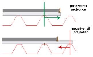
Rail projections are only possible at edge modules. The length of the rail pieces depends on the position of the clamping point to the next fastener. The rail length determined in the static calculation (min/max) must be transferred to the roof accordingly.
