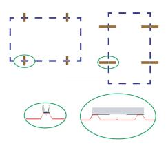
Mark the mounting position of the short profiles on the trapezoidal metal raised beads dependent on the module orientation – portrait or landscape, right-angled or on the raised bead – and the clamping areas specified by the module manufacturer. A gap of min. 10 mm must be maintained between the modules at the short frame side.
