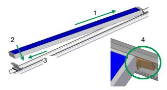
Place the module onto the top insertion rail and push it up (1). Then lower the module onto the bottom insertion rail (2) and push it down against the insertion rail (3). Mount the next modules following the same principle, the gap between the modules must be min. 3 mm.
