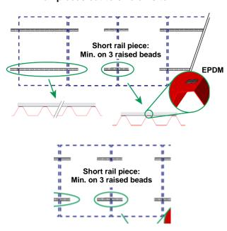
Mark the mounting axes of the rail pieces on the trapezoidal metal raised beads dependent on the clamping areas specified by the module manufacturer. Mark the position of the module clamps on these axes. Determine the length of the rail pieces from the Solar-Planit calculation dependent on the clamping position (taking into account MV 3.2 and 3.3) Glue EPDM sealing strips to the raised beads in the area of the rail pieces, fix the rail pieces to each raised bead across the rail piece length.
