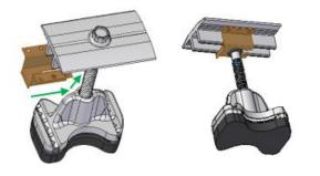
Push the contact latch on the sliding plate over the vertical webs of the middle clamp up to the screw.
