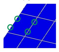
The modules must then be attached to the rails using end clamps and middle clamps – this applies analogously also to mounting the modules in landscape.
