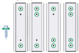
The static calculation in the system planning defines the number of fasteners required for mounting modules in landscape.
