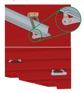
Position the trapezoidal sheet bracket with the aid of the mounting tool (1) on the insertion rail in the inclination of the raised bead with downward pressure.
