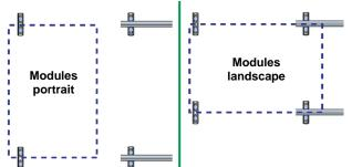
To improve ventilation behind the modules the modules can be mounted on short profiles.
