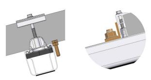
Prior to mounting modules in portrait, the module slip guards must be fitted to the frame holes above the bottom rail position (MV 3). For mounting modules in landscape module slip guard sets must be inserted at the lowest module row.
