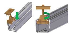
Insert the middle clamps or end clamps at the clamping position from above into the rail chamber. Then turn the rail nut in the rail and push the module clamps towards the module frame.
