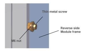
Push the nut over the screw and screw the thin metal screw into the module frame without predrilling.
