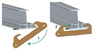
Place the insertion rail onto the EPDM strips, maintain 10 mm gap at the rail joint, Hook the trapezoidal sheet bracket into the rail on one side, feed it below the rail (1) and hook it in on the other side (2). The trapezoidal sheet brackets must be hooked into the insertion rail on both sides.
