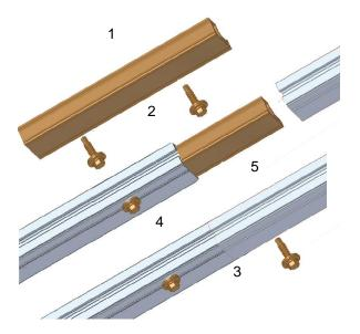
Push the connector (1) half way into one of the rails to be connected (2) and secure it there with a drilling screw in the lateral drilling groove. Next push the other rail completely onto the connector until both rail ends touch (3) and also secure with a drilling screw. Maximum uninterrupted rail length 13 m, then install expansion joint.
