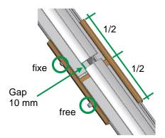
Module mounting: insertion system
