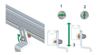
Place the N-rail near the slot against the roof hook (1). Rotate the screw head by 90° until the slot bolt is anchored in the groove (2). Align the rail (3) to compensate for roof irregularities and to make the ribbing engage with each other, then tighten. The roof hook can also be connected to the rail connector in the joint area. For mounting in the cross rail arrangement the top rail is attached using the Cross rail connector set N (MV 3).
