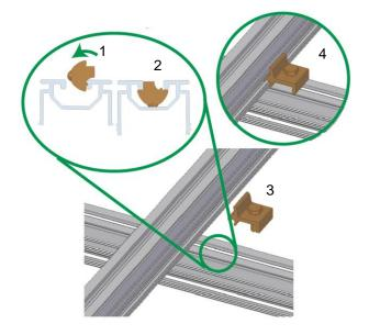
Insert the slot nut into the rail groove (1 and 2). Attach the fixing clamp with the screw (3) to the slot nut and push it against the upper rail (4) until the Cross rail connector set N M8 engages with the mounting flange.
