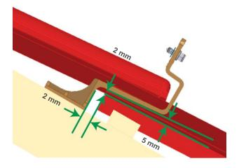
The minimum gaps between the bottom tile and support bracket must be adhered to. Align the roof hook to the centre of the rafter.
