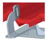
Interlocking tiles / concrete roof tile At the exit area of the roof hooks carefully make a cut-out with the angle grinder.
