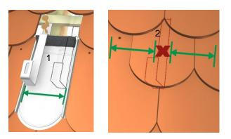
Align the roof hook in the centre of the rafter (1). Observe the permissible distances to the screws at the rafter edge. Do not place screw joints and support point at the locations of a joint (2). Screw in wood screw without predrilling.
