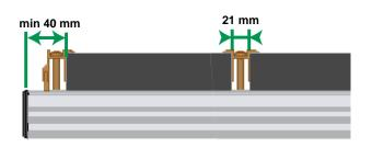
Fully assemble the end clamp, insert the spacer to do so (1). Place the module clamp onto the N-rail and press it on (2) until the slot nut engages with an audible "click" in the groove channel (3).
