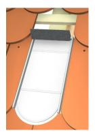
Determine the position of the sheet metal tile. Replace tile with plain tile sheet – the metal sheet edges are below the adjacent tiles – and secure with screws, then glue on foam wedge.
