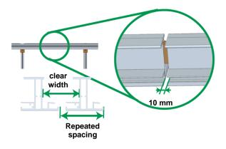
Attach the insertion rail Plus to the N-rails with Cross rail connector set N IR M8 as the insertion rail. Insert the connector for insertion rail Plus up to the stop and push the second rail with a distance of 10 mm over the rail connector.
