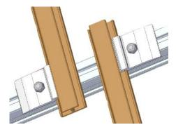
Attach the support rail IR with the Cross rail connector set N IR M8 - the support rails must be fitted parallel to the insertion rails and must be offset on the N-rail in the overlap area.
