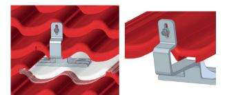
Interlocking tiles / concrete roof tile At the exit area of the roof hooks carefully make a cut-out with the angle grinder.
