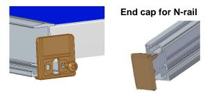
Centre the rail connector over the fitted rail and tighten the first threaded pin. Insert the rail to be connected into the connector, gap between the rails 10 mm, tighten the second threaded pin without play. MV 1 must be complied with for the mounting of the insertion rail Plus rails.
