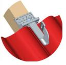
Insert roof hook with the bracket positioned in the trough of the roof tile. Mark the top tile and, if necessary, the bottom tile at the roof hook exit point. If the distance to the tile cannot be maintained, either use additional support plates (optional component) or roof hooks ZD 633. For plain tile covering proceed according to MV 2 (clamping system mounting version).
