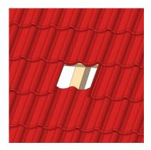
Expose the rafters by removing the tiles.
