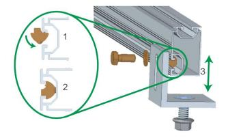
Position the slot nuts in the groove of the Nrail (1+2). Align the rail to compensate for roof irregularities (3) and to make the ribbing engage with each other, then tighten.
