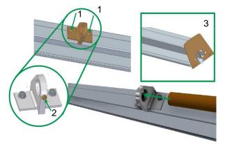
The brackets must be fitted with two drilling screws (1) to the insertion rail Plus. Position the rounded pipes centred and secure them with the grub screw (2).
