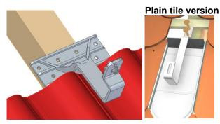
Insert roof hook with the bracket positioned in the trough of the roof tile. Mark the top tile and, if necessary, the bottom tile at the roof hook exit point. If the distance to the tile cannot be maintained, use additional support plates (optional component). For plain tile covering follow the instructions in the clamping system mounting versions (MV 2).
