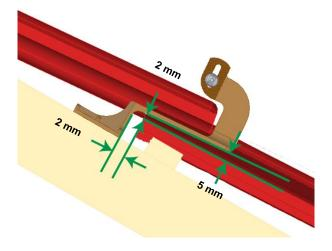
The minimum gaps between the bottom tile and support bracket must be adhered to. Align the roof hook to the centre of the rafter.
