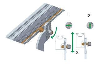
Place the N-rail near the slot next to the roof hook (1), rotate the screw head by 90° until the slot bolt is anchored in the groove (2), align the rail (3) to compensate for roof irregularities and to make the ribbing engage with each other, then tighten. The roof hook can also be connected to the rail connector in the joint area.
