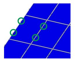
The modules must then be attached to the rails using end and middle clamps.
