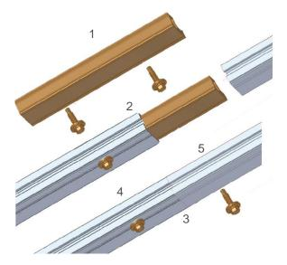
Push the connector (1) half way into one of the rails to be connected (2) and secure it there with a drilling screw in the lateral drilling groove. Next push the other rail completely onto the connector until both rail ends make contact (3) and also secure with a drilling screw. Maximum uninterrupted rail length 13 m, then install expansion joint.
