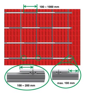
Distance between Aluminium round pipes at the end of the insertion rail in the corner area of the system max. 100 mm. Distance between round pipes min. 100 mm
