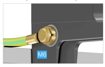
Screw the ground cable to the lower left side or lower right side of the ground connection (torque: 3.9 Nm). This requires an M6 screw, spring washer and washer. A toothed washer is **not** required.
