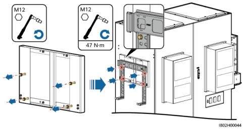
Figure 7-29 Installing a mounting bracket
