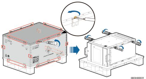
**Step 6** Install the operating handle on the battery pack, place the battery pack on the installation kit, and secure the battery pack.
