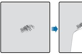
**Step 2** Dip a piece of cotton cloth into anhydrous alcohol and wipe the polished or damaged area to remove the dirt and dust. Then wipe off the anhydrous alcohol with a clean and dry cotton cloth
