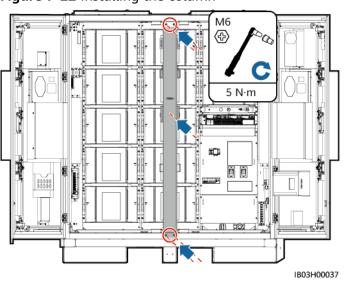
Figure 7-22 Installing the column
