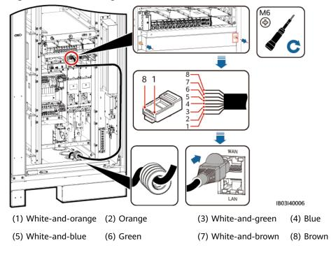
Figure 8-13 Connecting the FE communications cable
