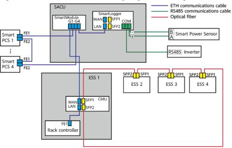
Figure 2-33 Communication networking diagram (fiber ring network)
