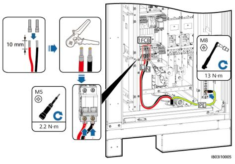
Figure 8-11 Connecting the AC power cable
