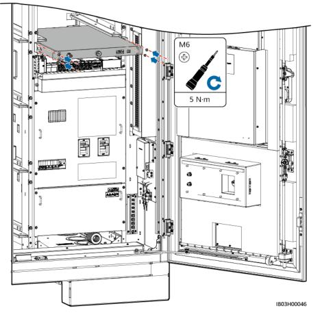
Figure 7-12 Installing the rack mounted fire extinguishing system
