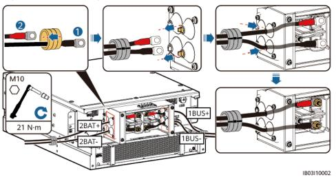
Figure 8-6 Connecting cables
