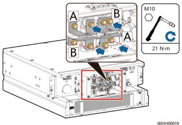
**Figure 7-24** Installing short-circuiting copper bars
