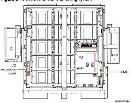
Figure 2-11 Position of the monitoring system
