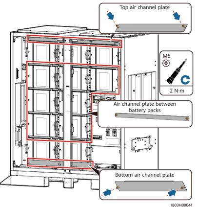
Figure 7-21 Installing air channel plates
