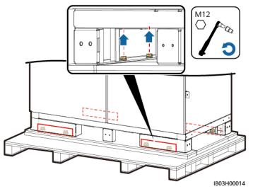
**Step 3** Install the baffle plate to the bottom of the ESS.
