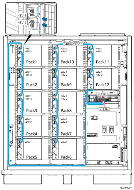
Step 3 Connect cables to the COM ports on the battery packs.
