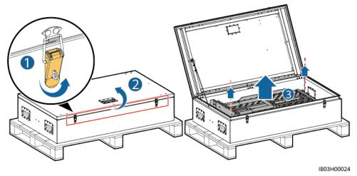
Figure 7-15 Taking out the installation kit
