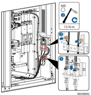
Figure 8-17 Connecting optical fiber cables
