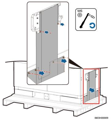
Figure 7-1 Removing the bottom baffle
