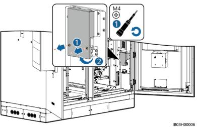
Figure 8-15 Removing external mechanical parts
