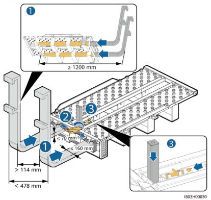
Figure 7-16 Assembling the installation kit
