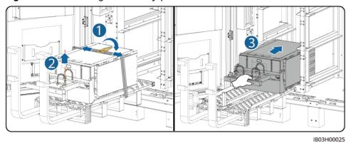
Figure 7-19 Installing the battery pack in the ESS
