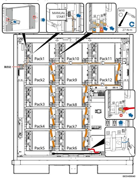
Step 2 Connect 48 V cables to the battery packs.
