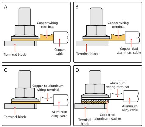
Figure A-1 Requirements on an OT or DT terminal
