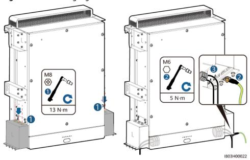
Figure 8-9 Connecting a ground cable
