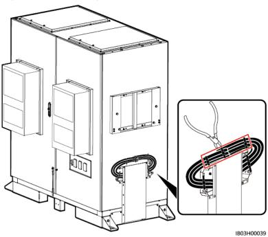
Figure 7-26 Removing bound cables
