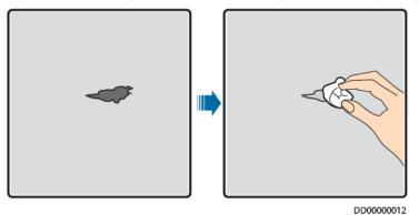
**Step 3** Paint zinc-rich primer on the damaged coat using a brush or paint spray gun.
