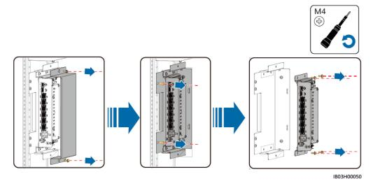
**Step 3** Install a new I/O expansion board.
