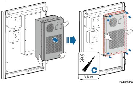
Figure 8-19 Installing a new air conditioner
