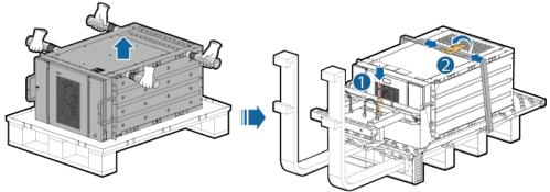
Step 11 Install the new battery pack in the ESS.
