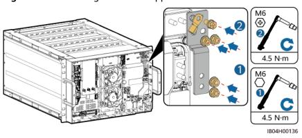
Figure 5-10 Installing the short copper bar
