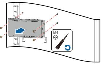
Figure 20-2 Removing the TCUE control box
