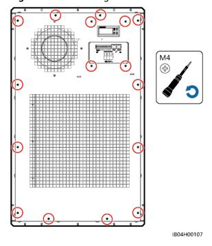
Figure 8-12 Removing the front cover of the air conditioner
