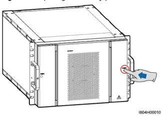
**Figure 4-1** Opening the battery pack covers
