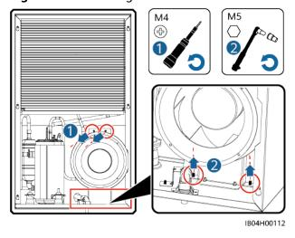
**Step 3** Remove cables from the quick connect port of the external fan, and remove the external fan from the support.
