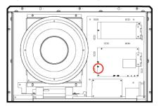
**Step 6** Remove the internal fan from the fixing plate.
