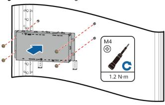
Figure 20-6 Reinstalling the TCUE control box
