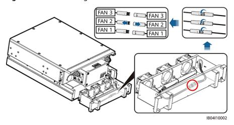
**Step 4** Remove cable ties from the faulty fan.
