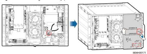
**Step 6** Remove the nuts from the management module.
