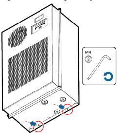
Figure 8-7 Removing security torx screws
