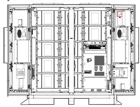
Figure 22-1 Position of the exhaust fan
