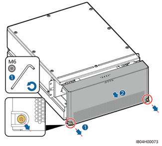
**Step 2** Remove screws from the fan tray, and then pull it out.
