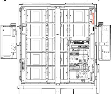
Figure 20-1 Position of the exhaust controller (TCUE)
