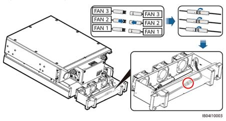
**Step 9** Push the fan tray into the slot and tighten the screw.
