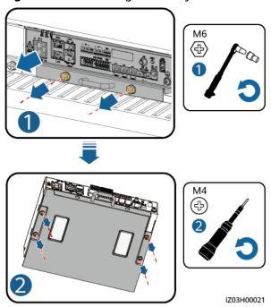
Figure 16-3 Removing the faulty CMU
