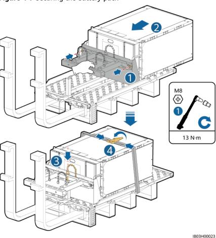
Figure 4-7 Securing the battery pack
