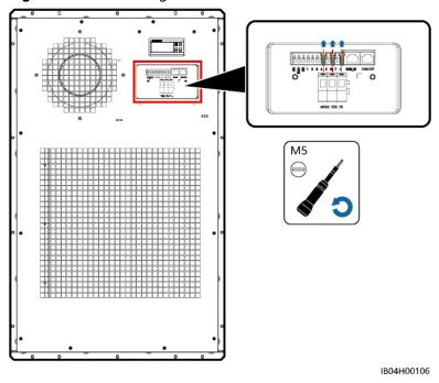
Figure 8-17 Removing air conditioner cables
