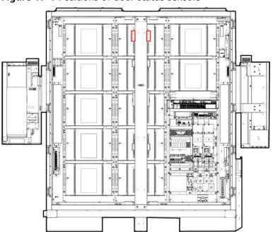
Figure 17-1 Positions of door status sensors
