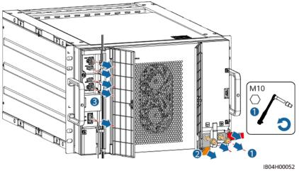
**Step 4** Remove screws from the battery pack.
