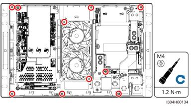
Figure 5-9 Installing the nuts
