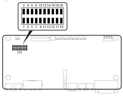
Figure 20-4 Positions of the jumpers on the TCUE control board
