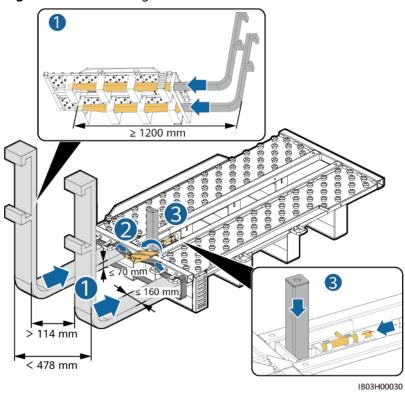
Figure 4-6 Assembling the installation kit
