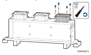
**Step 6** Install a new fan (FAN 1 is used as an example).
