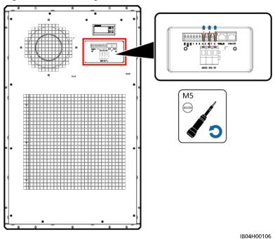
**Step 3** Remove the front cover of the air conditioner.
