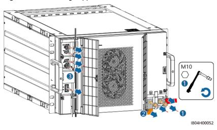
**Step 3** Remove the front panel of the battery pack.
