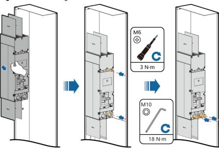
Figure 11-3 Installing a DC switch
