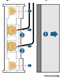
Figure 17-2 Removing the door status sensor
