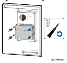
**Step 2** Remove cables from the air conditioner.
