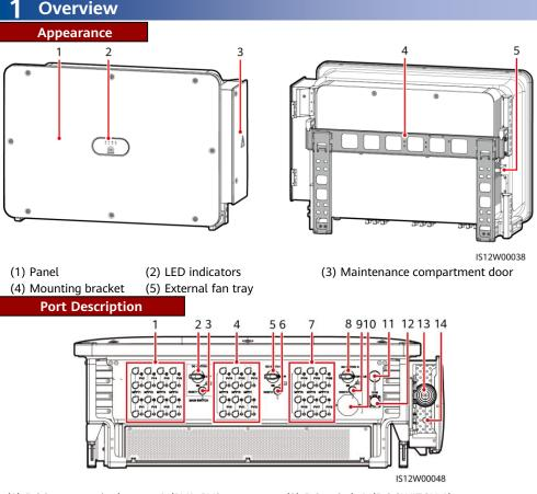
(1) DC input terminal group 1 (PV1–PV8, controlled by DC SWITCH 1)
