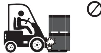
Inserted from the long side, the backrest is below the height of the package and there is no gap between it and the box, which can break the glass by pressing the internal modules.
