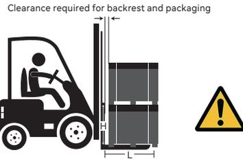
Forklift tines inserted from the long side (allowed, but not recommended).  $H >$  single trailer packing height,  $L >$  90% of pallet length.
