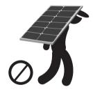
Do not move or handle the modules by dragging the junction boxes or cables under any circumstances, to avoid loosening of the connector (causing electrical hazards) or dislodging (causing damage to the product or personal injury).
