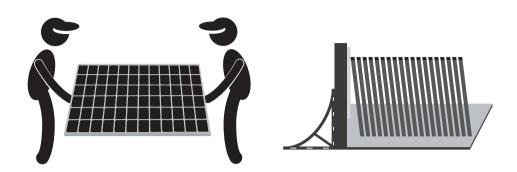
Lift the modules: two persons hold the two short sides of the module and lift the to it designated place simultaneously. Protective gloves must be worn during the unpacking process to avoid cutting hands. Do not touch the glass surface with fingers to avoid leaving fingerprints on the glass surface.
