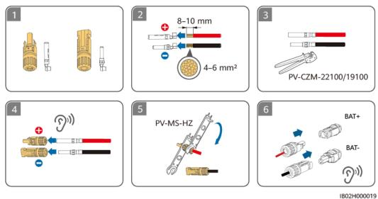
In a parallel system, connect DC power cables between the ESSs by referring to cable connections between the inverter and an ESS.
