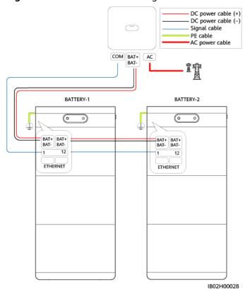
Figure 3-1 Cable connection diagram
