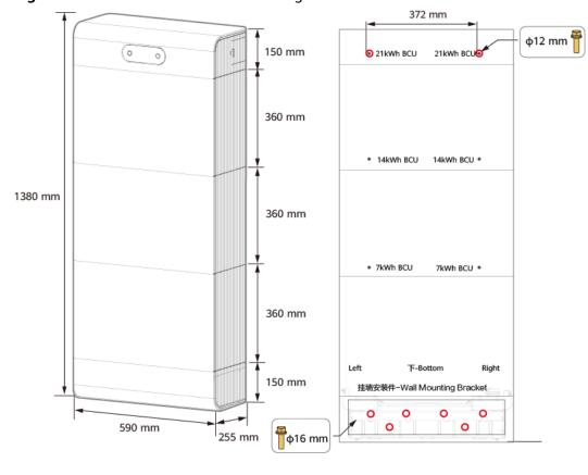
Figure 4-5 Dimensions for wall mounting
