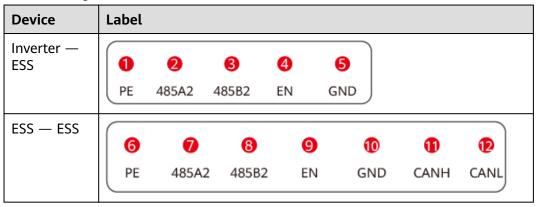
Figure 5-6 Signal port connections
