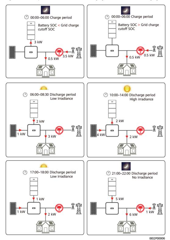
Figure 2-9 Example of TOU (00:00-06:00 charging and 6:00-24:00 discharging)
