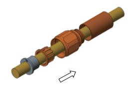
3. Strip the cable. Put the support sleeve on the cable, and plug the stripped cable core into the metal terminal.
