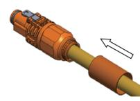
11. Remove the plastic cover before plugging it into the battery system.
