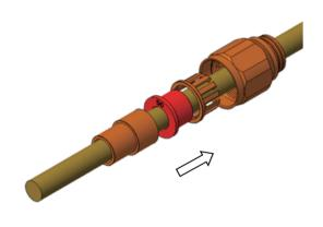
3. Strip the cable for 20 mm. And cover the stripped cable core with the metal terminal.
