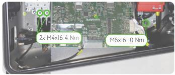
After a successful electrical installation, it is crucial to mount the protection cover (M4x16 Torque: 2,5 Nm) from the cable entry. If not installed properly, this can lead to significant damages on the charging station as it's not sealed hermetically.
